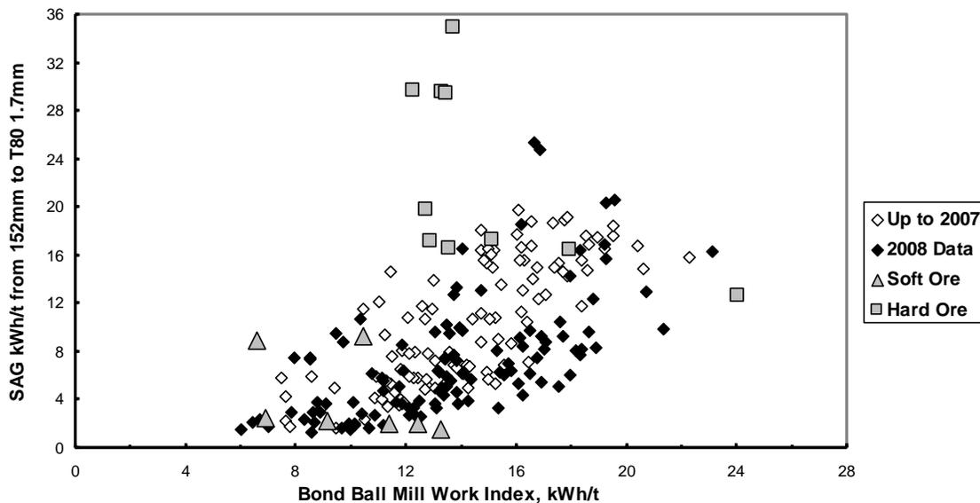
Figure 1 - Database SAG and Bond Data by Year - Including Soft and Hard Ore
