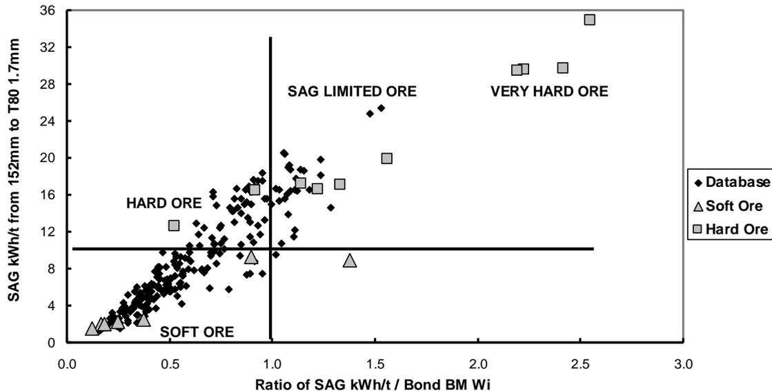
Figure 2 - SAG Pinion Energy Vs Ratio of SAG / Bond BM Wi, including Soft & Hard Ore
