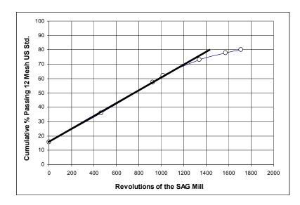
Figure 1 – Typical SAGDesign Test result
