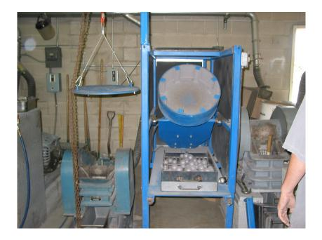
Figure 2 – SAGDesign Test Mill
