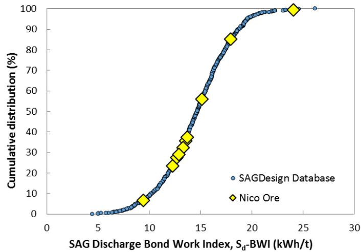
Figure 2 – SAGDesign Database: SAG Discharge Bond Results,  $S_d$ -BWI Vs Dist. %
