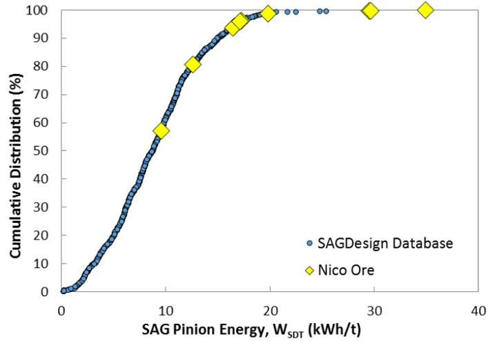
Figure 1 – SAGDesign Database: SAG Test Results, SAG Pinion Energy ( $W_{SDT}$ ) Vs Dist. %.
