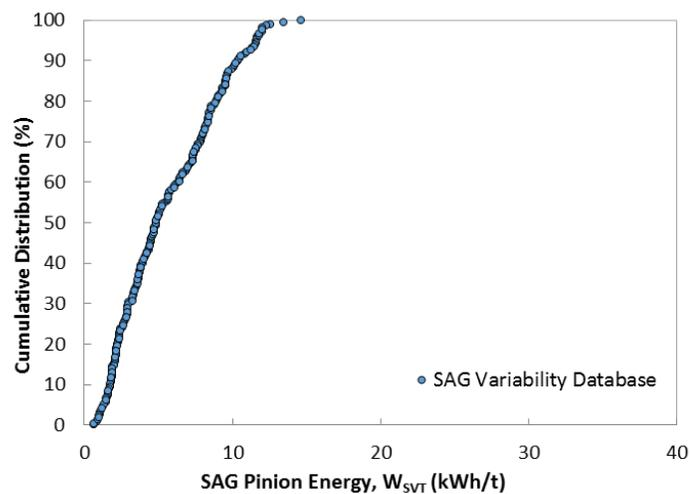
Figure 4 – SVT Database: SAG pinion Energy,  $W_{SVT}$  Vs Dist. %
