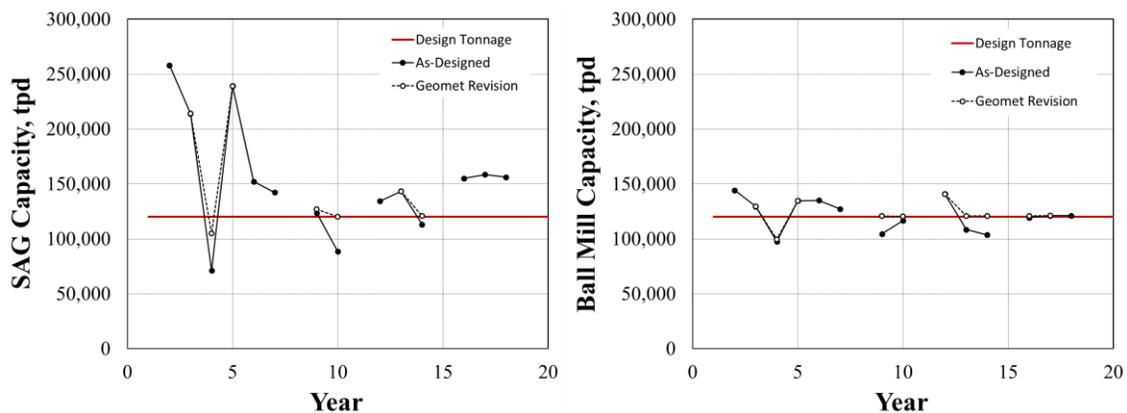
Figure 5: SAG and Ball Mill Capacity during Geometallurgical Scoping Study
